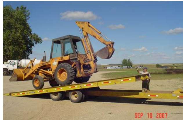
Use extreme caution in loading and unloading equipment and use a helper to guide you if possible.
