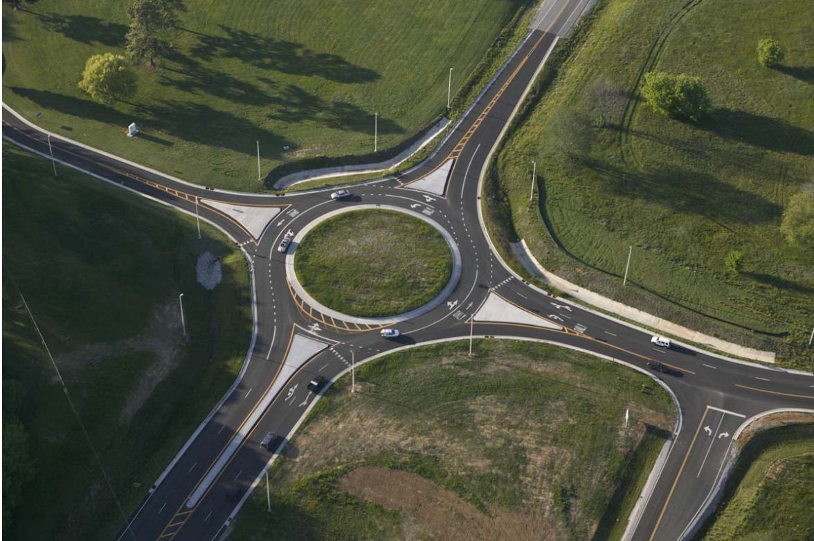
New pavement markings taken from the draft 2008 edition of the MUTCD offer guidance to unfamiliar drivers before entering the new multilane roundabouts.
