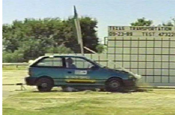
Crash-testing a work zone device (TTI).
